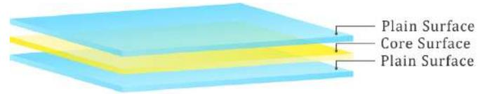
**KEY FEATURES**-SPARSHPET-DD is an optically high clear transparent film with high clarity low haze, high gloss plain surface on both sides. The film possesses good optical and surface properties, good friction, excellent transparency and dimensional stability.
